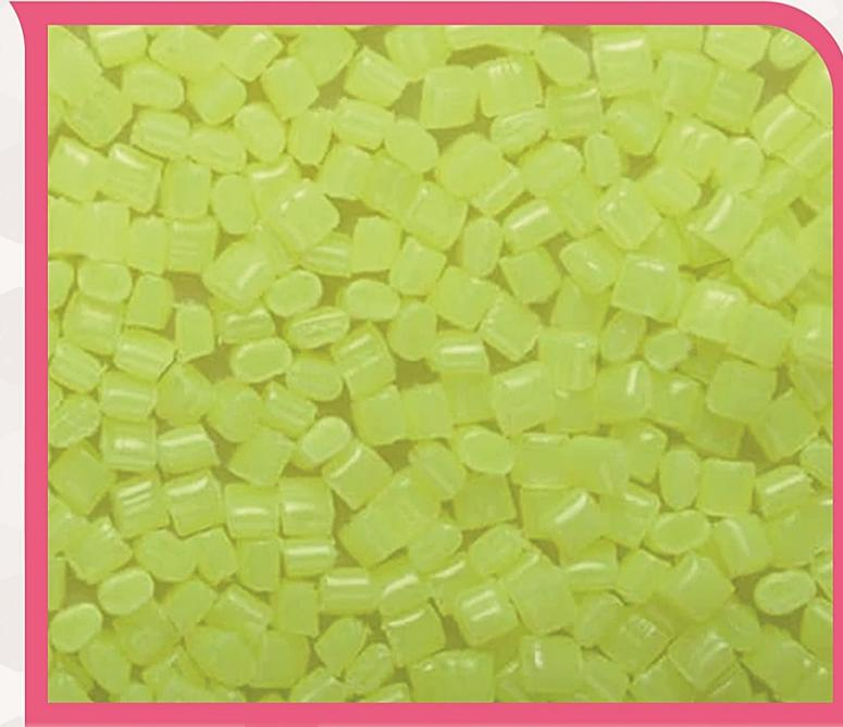
Antioxidants are used to protect polymers from degradation, both during processing (=short term stabilization) and during use (=long term stabilization). Polymer degradation generally results in gel formation and changing melt flow index, loss of mechanical and esthetical properties (crazing, gloss reduction, chalking), and discoloration.
