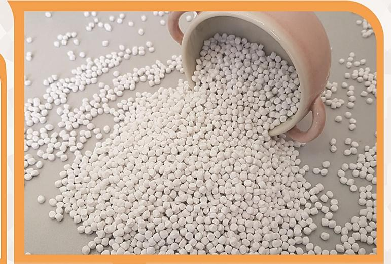
Natural polymers may lack the properties required by the customer, therefore, in order to improve the properties, polymers are mixed with each other or with other materials such as mineral additives such as Calcium carbonate. Polyethylene (PE) compound reinforced with calcium carbonate is used in the following industries
