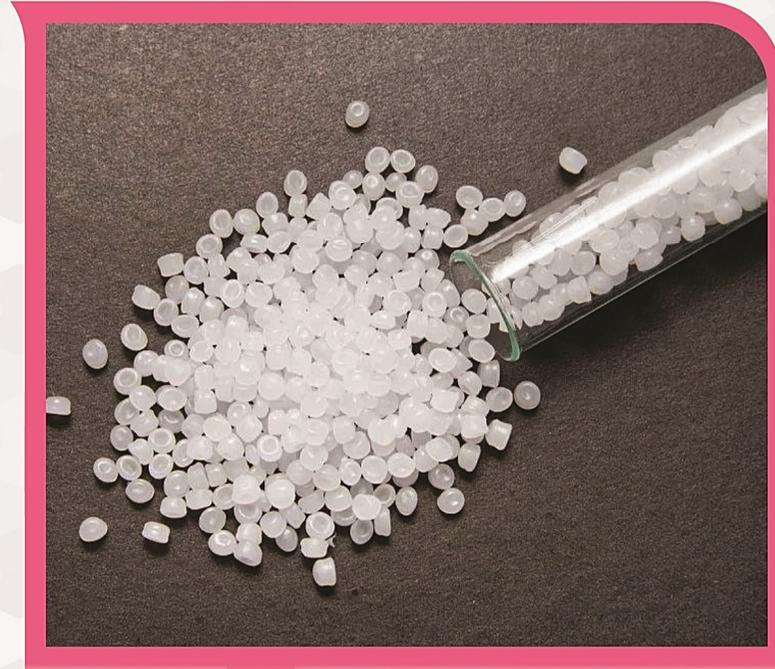
A slip agent is a large molecule with high molecular weight that's extremely slimy in melted form. Adding a slip agent decreases friction significantly, increasing the life of machinery and improving production rate.
